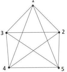
In the point-to-point connection, for **n** entities, we need **n(n-1)/2** links. All these links form a network. Networks with point-to-point links among all the entities are known as **Fully Connected Networks**. The number of links required in a fully connected network becomes very large even with moderate values of **n**.
